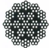
19 X 7 ROTATION RESISTANT WITH WIRE STRAND CORE
